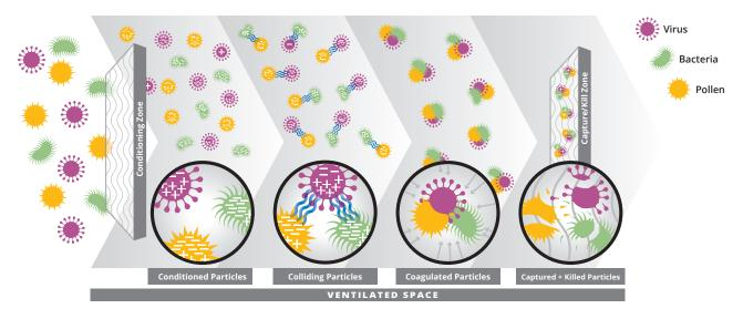
ACTIVE Particle Control Technology conditions particles and pathogens, induces collisions leading to particle coagulation, and then once collected on the capture media kills all biologic matter.
